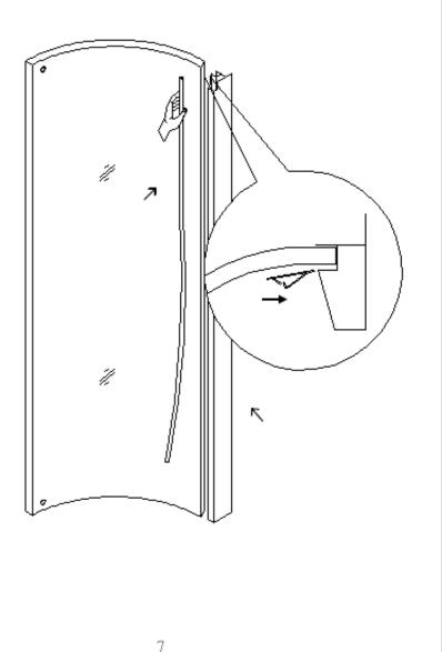
Fixing the fix glass door to the aluminium file with the screw(4\*12). then put the [H] aliminium to the glass. Then install the belt.
