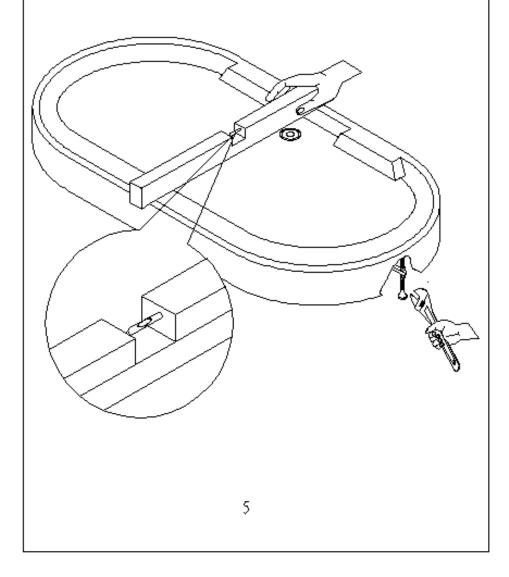
Install the hings with the fix glass.
