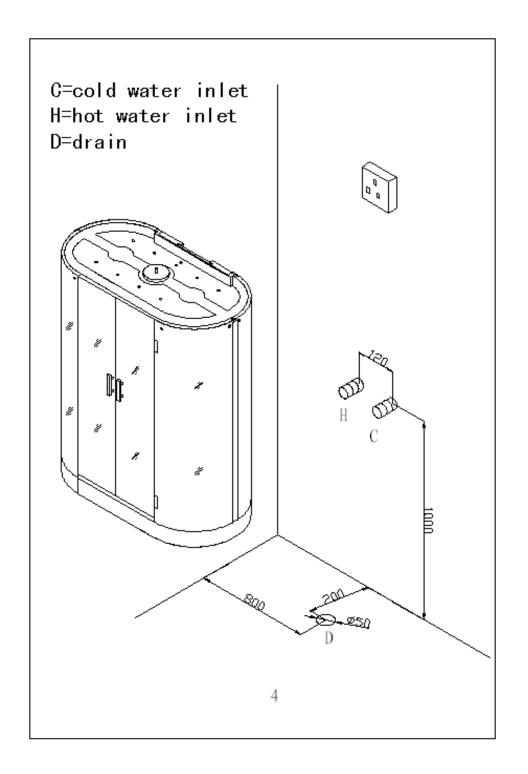
Put the base at the right place, adjust the feet and tighten the screws.
