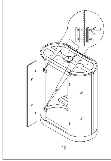
Put the fixer to the glass on the bottom with screws (4\*20) and screws cap. then use the screws (5\*20) at last
